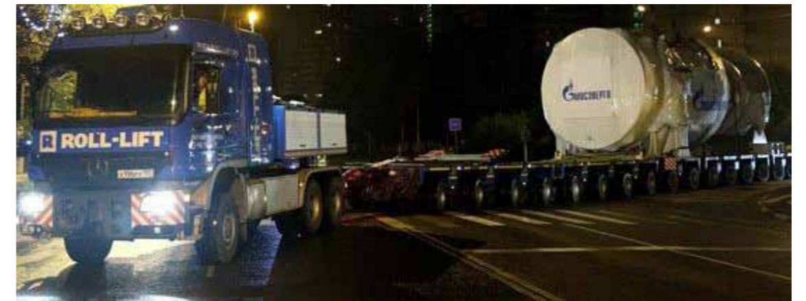
Fig. 12. Delivery of a new gas turbine to the CCGT-420 unit at TPP-20
