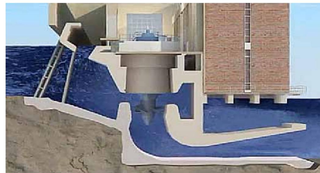
Fig. 40. Hydro turbine operation scheme with Lesogorskaya HPP as an example
